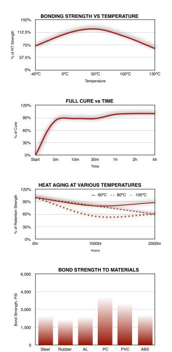
Figures are tested to ASTM 4501. Results may differ with varying application bonding areas, contact surface areas, coatings and material grades. etc.
