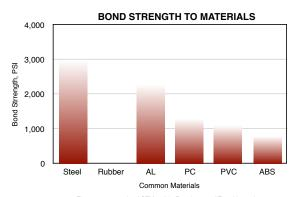
Figures are tested to ASTM 4501. Results may differ with varying application bonding areas, contact surface areas, coatings and material grades, etc.
